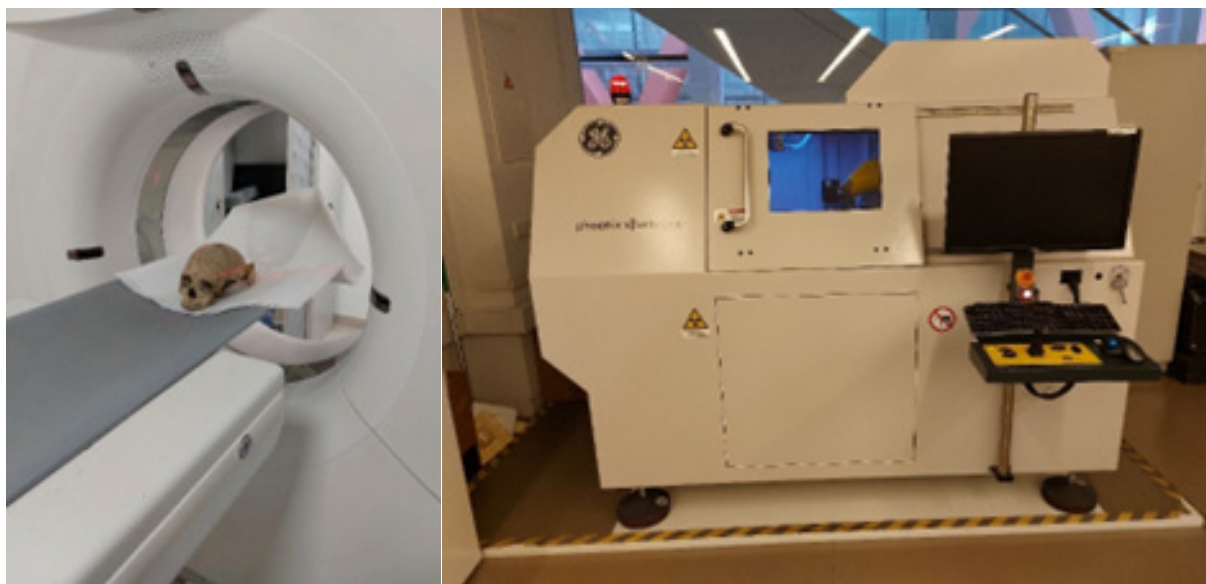
Figure 2. (a) The hypogeum skull, one of the skulls in this project, being CT scanned in Malta prior to initiating diagnostics abroad; and (b) the CENIEH nCT scanner used to image the carbonized dough fragments (see bottom left inset).
